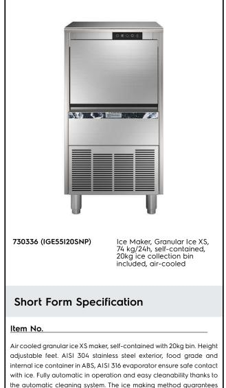
continuous and reliable production. Electronic board controls the set parameters and sensitive touch-press panel with 2 speed regulation of ice production. Bin with internal corner for easy cleaning and it is fully insulated. Supplied with flexible water supply, drain hosed and scoop. Hydrocarbon refrigerant gas R290 for the lowest environmental impact.
